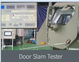
**Use** Door Slam Test&Measurement
