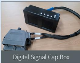
**Use** Dual Signal Monitor for High Speed Train
