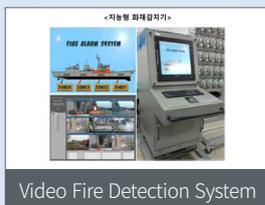
**Use** It detects a water leak, flame, and explosion by analyzing a CCTV real-time input image./It detects fire early and in broad areas
