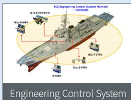
**Use** Display and process information for each device on the vessel/Provide operation, control, and observation functions of the propulsion system
