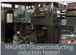
MAGHEET(Superconducting induction heater)
